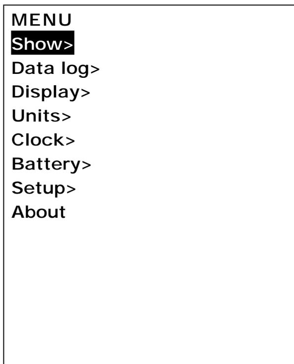
The first menu item “Show” is highlighted, different menu items can be highlighted using the **↑** and **↓** buttons. The wanted action is done by highlighting the appropriate menu item and pressing the **Set** button. To abort without doing anything press the **X** button. In some cases a further sub-menu is displayed with more choices.
